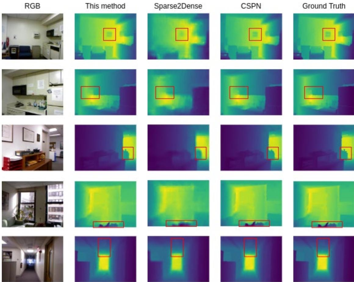
**Figure 2.5** Qualitative result of the proposed active fusion model. Sparse depthmap is collected by composing three different sampling layers: 1) saliency map-ping with density downsampling, 2) edge detecting, 3) grid-sketch distributing. The composing depth map (second column) contains 6, 000 pixels, focusing on “most important” parts of an image.
