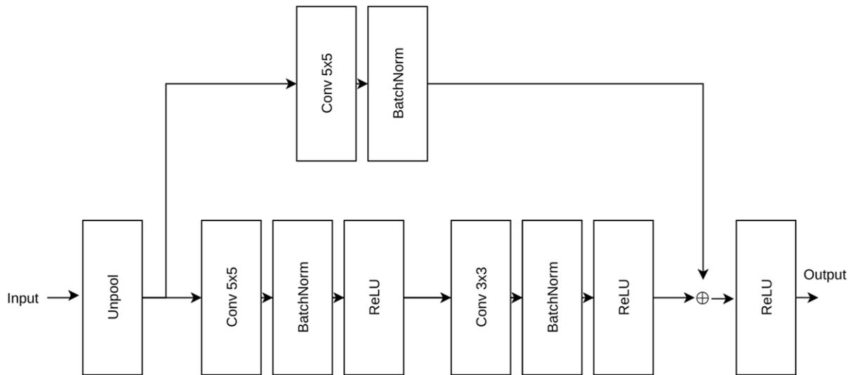
**Figure 2.3** Structure of the bottleneck residual block
