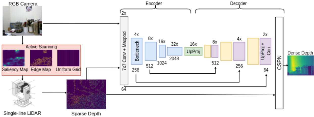
**Figure 2.1** The overall framework of our depth completion network. Given a RGB-D input ( $304 \times 228 \times 4$ ), the tensor first goes through  $7 \times 7$  convolutional layer, following with 4 downsampling steps and 4 upsampling steps. Sparse depth map is directly mapped as affinity to guide the depth completion. Notice the integration of the third generation LIDAR system as described in the previous chapter.
