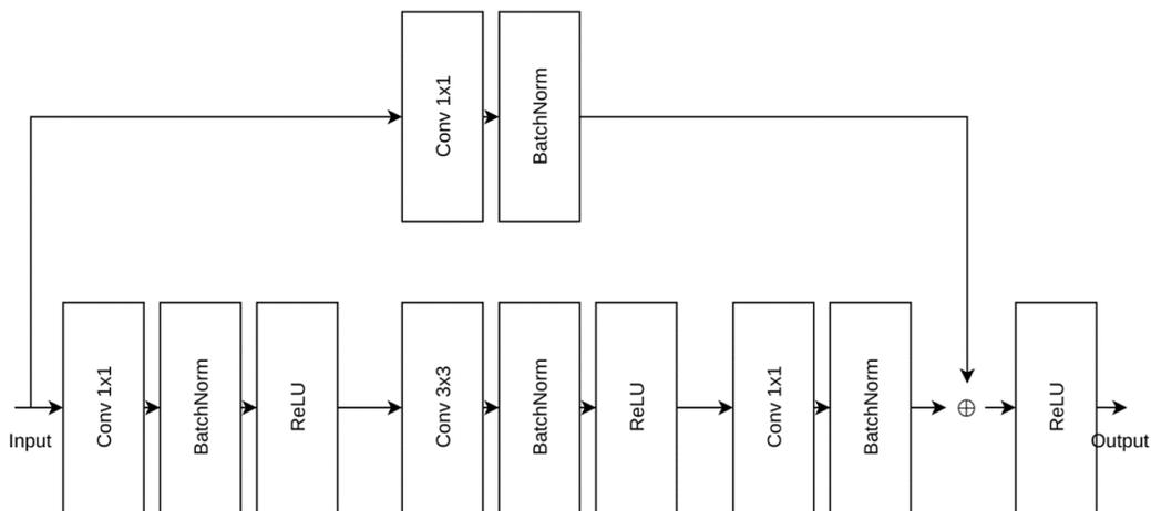
**Figure 2.2** Structure of the bottleneck residual block
